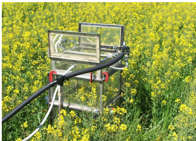
Figure 1. A nitrous oxide collection chamber at Cunderdin.
